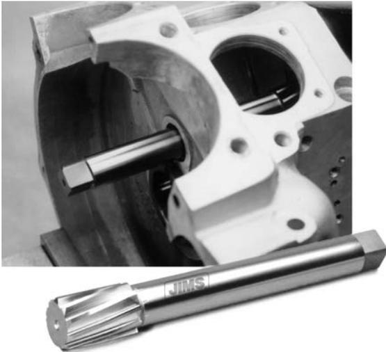
1. To install a new outer cam bushing use JIMS Tool no.1012-70TB bushing installer.
