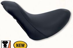
Bolt-on solo seat with black Naugahyde cover and steel base plate with a black paint finish.
