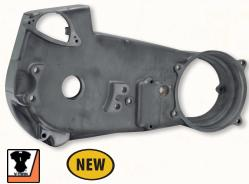
This polished inner primary cover has the hole for the mid shift control lever as OEM. It features a 9-hole pattern for the outer cover to bolt to. If your outer cover only has 8 holes the 9th simply isn't used. The casted-in reinforced webbing makes this inner primary very strong. Note that the polishing is not up to the Zodiac standards and it is therefore recommended to have the cover painted or powdercoated.
