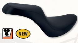
Bolt-on duo seat features a frame hugging design, black Naugahyde cover and steel base plate with a black paint finish. Seat is 13" (33cm) wide for the driver and 8 3/4" (22cm) wide for the passenger. Installation may require the separate purchase of ZPN 098010 seat bracket.
