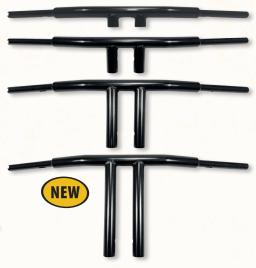
These handlebars are 1 1/2" (38mm) in diameter with 1' (25.4mm) ends to accept stock controls. Bars are dimpled and pre-drilled to accept internal wiring. They bolt to the upper fork tree with 1/2"-13 UNC bolts on most Harley's with a 3 1/2" (89mm) center to center. Bolts are not included. Handlebars are ready to take Throttle-by-Wire, as well as regular cable throttle.
