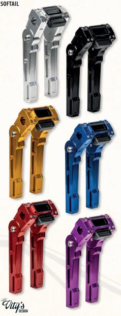
Billet aluminum risers in 8" (20cm) or 10" (25cm) high with an adjustable head and one-piece top clamp for use with handlebars that are 1" in diameter at the riser mounts. Comes complete with M12-1.5x70mm riser bolts. Top clamp is ready to take the 0EM digital instrument cluster.
