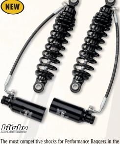
market. They are easily adjustable with an exposed remote reservoir featuring a 12-click compression knob, 5-position rebound adjustment lever and fine thread preload nut to help setup the ride for maximum performance. These extra long shocks for 2014 to present Touring models increase the ride height drastically but note that the wheel axle nut will sit lower and will contact stock length exhausts. Install with aftermarket exhausts that end before the axle nut.
