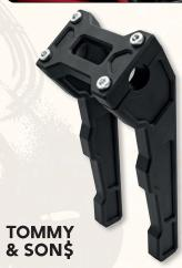
Billet aluminum risers with a black anodized finish are sold in sets for left and right. Risers are 10" (25.4cm) high and designed for 1" diameter handlebars. They are to be mounted using the stock riser bolts. Riser bolts are also available separately.
